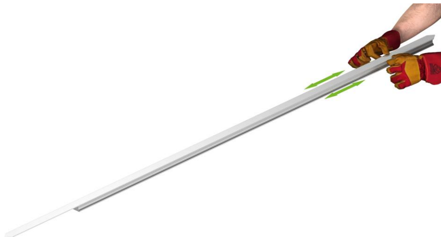
Fig. 5.28: Clamp on cover strip approx. 3 cm
